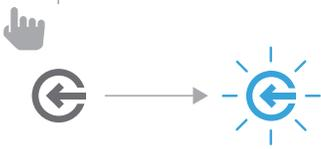
2. Use the device's Bluetooth pairing menu to pair it with the Harman Kardon Aura Plus. The unit will appear as **HK Aura BT** in the list of Bluetooth available devices. When the Harman Kardon Aura Plus's source button LED illuminates blue constantly, it is paired with the device and you can stream audio via Bluetooth from the device to the Harman Kardon Aura Plus.
